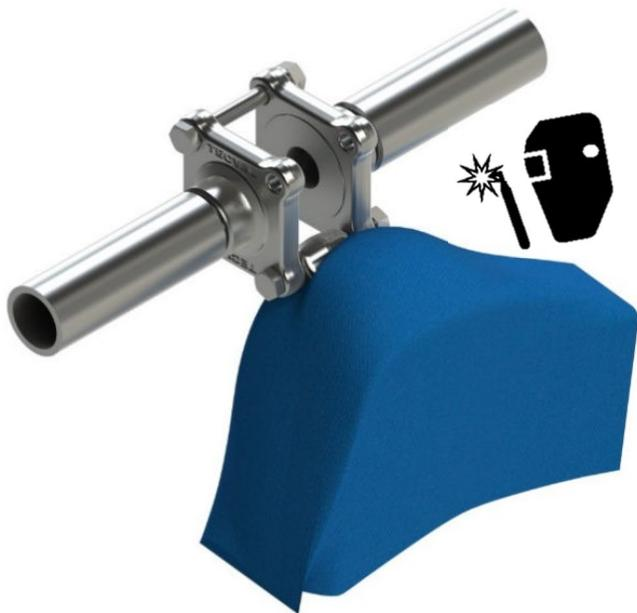
**8** Cooling processes. Reassemble O'ring Seat
