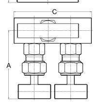
Maintenance Adjustment of the packings may be necessary during the working life of the manifold. The operation consists of turning the nuts (3) clockwise. Manifolds with long no-working period may have a harder initial operating torque.
