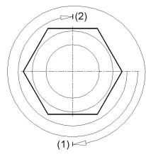
**Tecvalok** connections can be disconnected and reconnected repeatedly without loss of tightness, proceeding as follows: 1.- Before disconnecting, mark the position of the nut in relation to the body of the connector. 2.- To reassemble, use a wrench to tighten and bring the nut to the original position. 3.- Tighten the nut with the wrench only gently until there is a slight increase in torque. Then stop. The union will once again be secure and tight.
